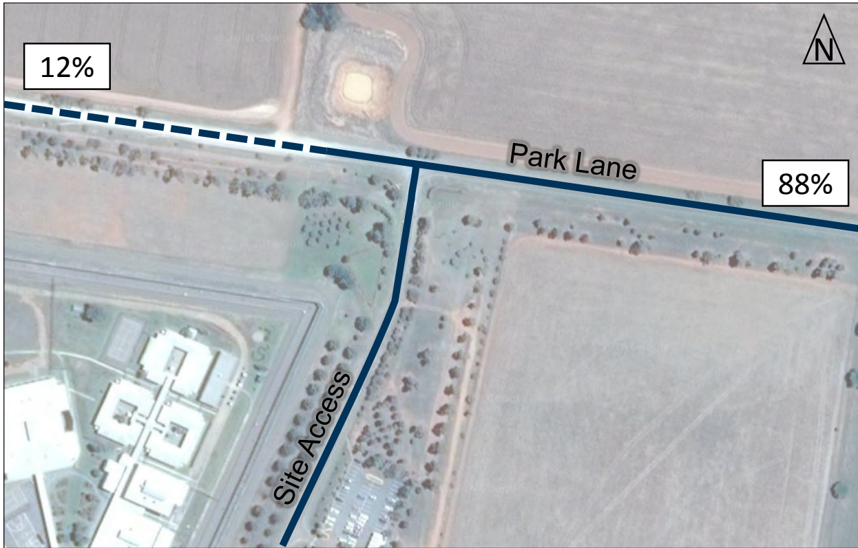
Figure 6 Distribution of Junee Correctional Centre Traffic
